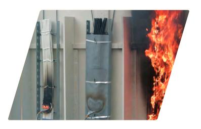
Comparison of fire damage to cable support systems (from left to right):
