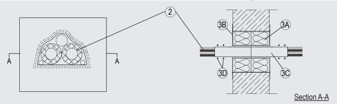
System tested with a pressure differential of 2.5 Pa between the exposed and the unexposed surfaces with the higher pressure on the exposed side.
