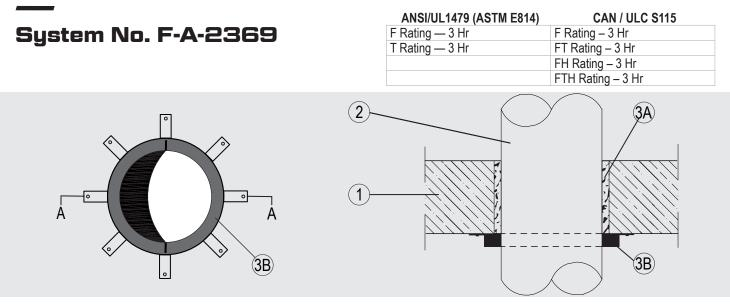
System tested with a pressure differential of 2.5 Pa between the exposed and the unexposed surfaces with the higher pressure on the exposed side.
