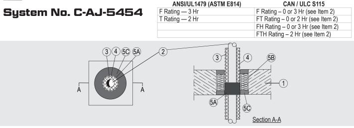
System tested with a pressure differential of 2.5 Pa between the exposed and the unexposed surfaces with the higher pressure on the exposed side.
