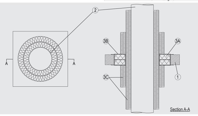
System tested with a pressure differential of 2.5 Pa between the exposed and the unexposed surfaces with the higher pressure on the exposed side.
