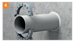
A suitable fire protection collar must be utilised.
