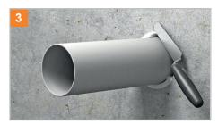
Before assembling the fire protection mortar, the remaining gaps between wall or floor and the inserted pipe are to be filled completely with dimensionally stable, non-combustible building materials, e.g. concrete, cement or gypsum mortar (class A1 or A2-s1,d0 according to EN 13501-1.
