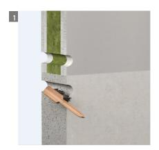
Clean the reveal and remove all loose parts.
