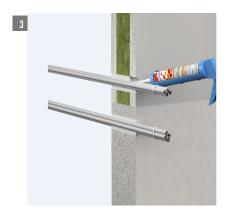
The remaining annular gap (joint betweet cable and component, width 0 - 10 mm) and the guessets in between cables as well as joints between cables and the component must be filled with intumescent FLAMRO DSB at building component's thickness.
