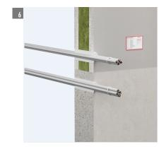
The penetration seal is to be labelled permanently with an identification sign. Finally clean work space.
