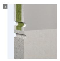
The gap between reveal and stands is to be sealed by inserting 100 mm of insulation of classification A1 or A2 according to EN 13501-1 inside the gap.
