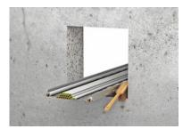
2. In walls the intumescent strip KERAFIX® Flexpan 200 NG-A (width: 50 mm) must be glued onto both side edges and centrally onto the top edge of the seal. In floors the strip must be glued onto all edges of the reveal while being flush with the lower side of the floor. If possible, insert the first layer of pillows below the cable bundle or the cable tray.
