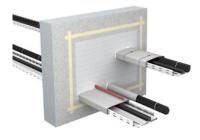
6. Label the penetration seal. Fill out the label neatly and attach it firmly next to/above (not on!) the penetration seal.
