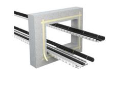
Cut mineral fibre boards to size and produce cut-outs for the installations. Coat the edges of the boards with PYRO-SAFE<sup>®</sup> FLAMMOTECT-A and insert the boards into the component.
