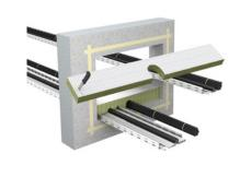
3. Seal remaining openings tightly with mineral wool or with PYRO-SAFE<sup>®</sup> FLAMMOTECT-A.
