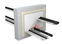
5. Apply final coating with PYRO-SAFE® FLAMMOTECT-A 4. Wrap cables, cable bundles and cable support structures with PYRO-SAFE® DG-CR 1.5.
