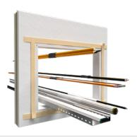
4. Cut mineral fibre boards to size (make cut-outs for the installations).
