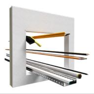
Mask the opening with crepe tape on all sides, keeping 20 mm distance to the edge. Coat the cables with PYRO-SAFE® FLAMMOTECT-A.
