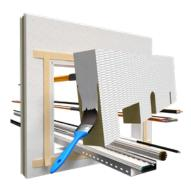
6. Seal the remaining opening / joint gaps with mineral fibre or fill with PYRO-SAFE® FLAMMOTECT-A.
