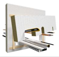
Coat the edges of the mineral fibre boards with PYRO-SAFE® FLAMMOTECT-A and firmly place boards in position.
