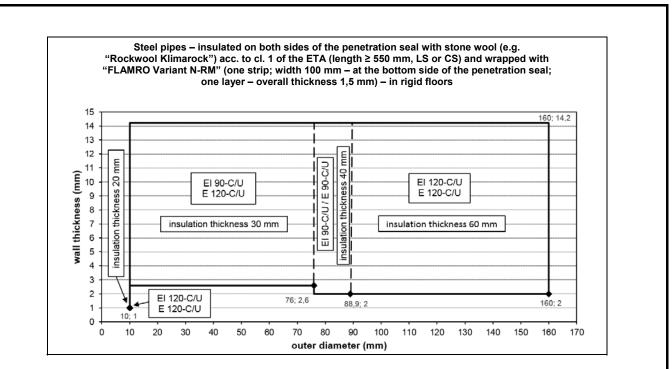
Note: The given graphs and therein enclosed fire resistance classes according to EN 13501-2:2007+A1:2009 are only valid for metal pipes according to clause 2.1 of the ETA.
