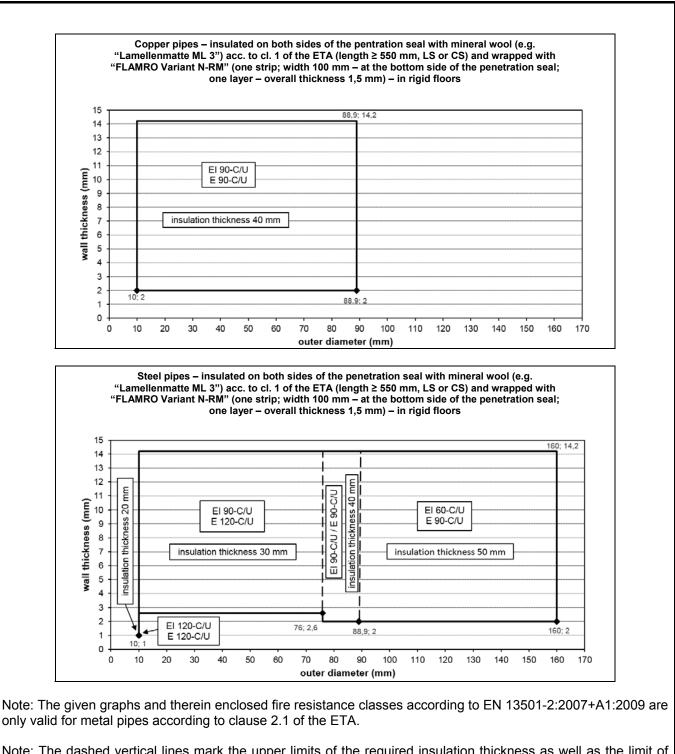
Note: The dashed vertical lines mark the upper limits of the required insulation thickness as well as the limit of the fire resistance classes.
