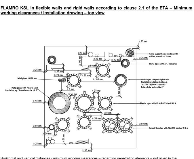
Horizontal and vertical distances / minimum working clearances – regarding penetrating elements – not given in the installation drawing have to be  $\geq$  100 mm in practice.
