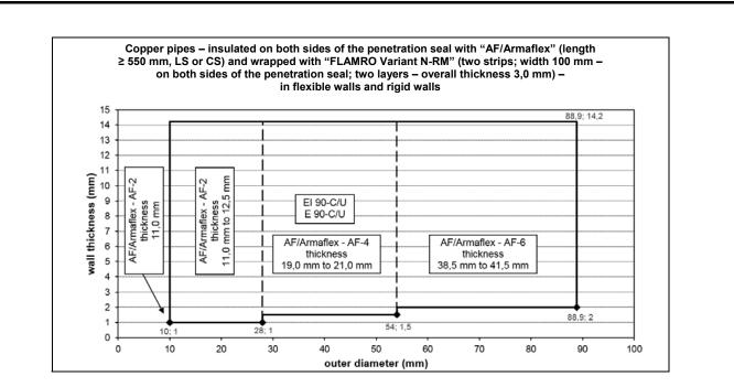
Note: The given graphs and therein enclosed fire resistance classes according to EN 13501-2:2007+A1:2009 are only valid for metal pipes according to clause 2.1 of the ETA.
