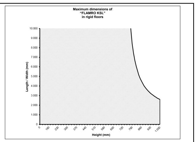
The maximum height of the penetration seal in rigid floors is 1000 mm.
