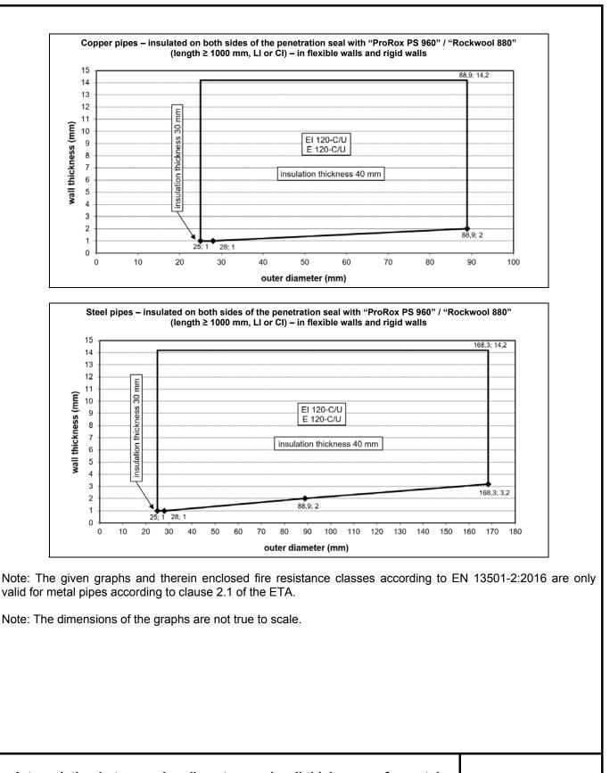
Interpolation between pipe diameters and wall thicknesses for metal pipes according to clause 2.1 of the ETA in flexible walls and rigid walls
