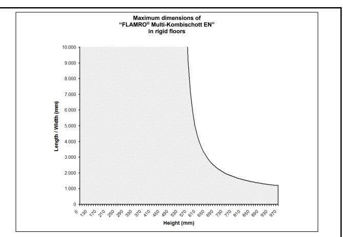
The maximum height of the penetration seal in rigid floors is 970 mm.
