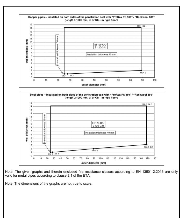
Interpolation between pipe diameters and wall thicknesses for metal pipes according to clause 2.1 of the ETA in rigid floors
