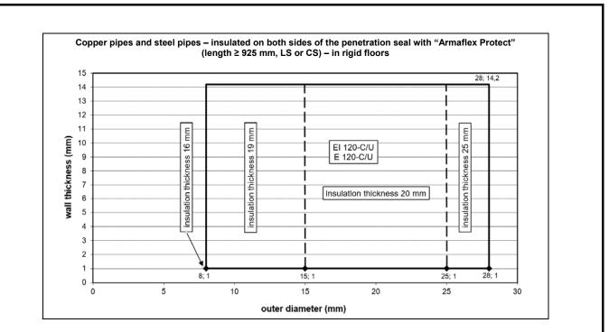
Note: The given graphs and therein enclosed fire resistance classes according to EN 13501-2:2016 are only valid for metal pipes according to clause 2.1 of the ETA.
